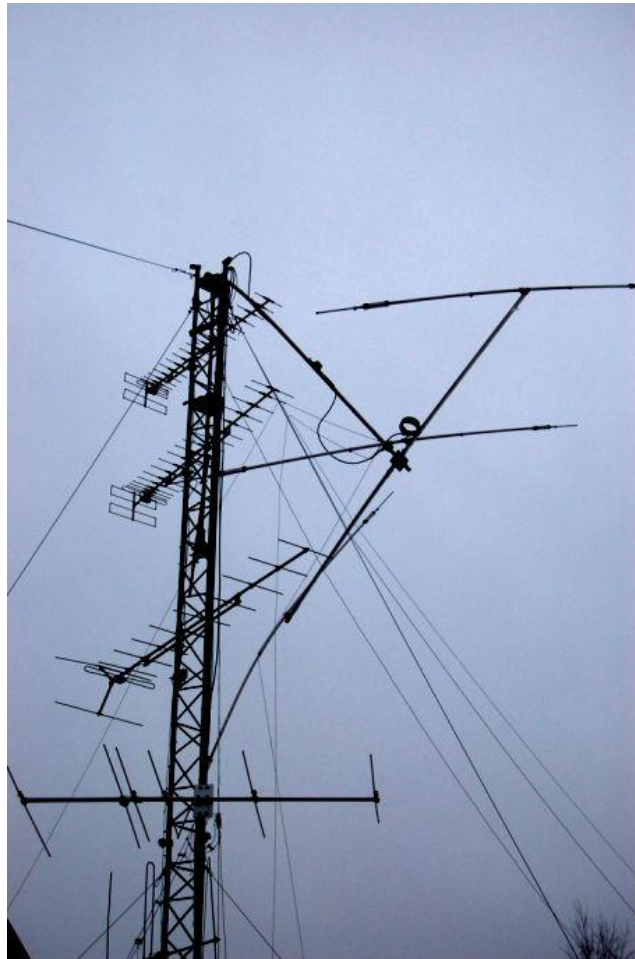
Jarmo, OH2GJL uses a tilting system to control the take-off angle.
