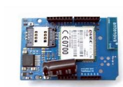
■ **Arduino GSM Shield**
