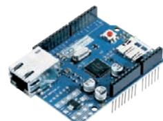
■ **Arduino Ethernet Shield**
