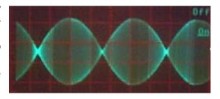
The picture shows the waveform of a well adjusted PSK31 signal, which resembles the waveform of a two-tone test, used for measuring PEP power in SSB.
