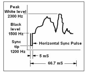
each line are 5ms in length and at the end of each frame 30ms in length.
